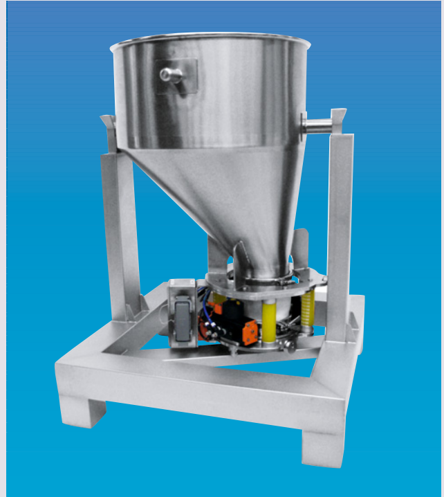
Silo with active valve – depending on the operation procedure it may be convenient to install the active valve at the vessel and the passive valve at the machine (in this case fixed to a mill).
